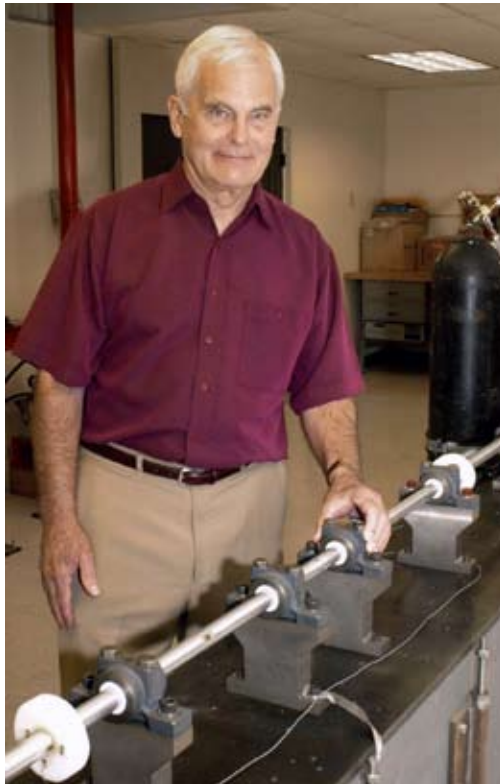
Dr. Ulric Lindholm with a present-day SwRI Split-Hopkinson Pressure Bar apparatus. In the 1960s, he and coworkers developed a technique that allowed direct generation of the complete dynamic (high-rate) stress-strain curve in a single experiment.
