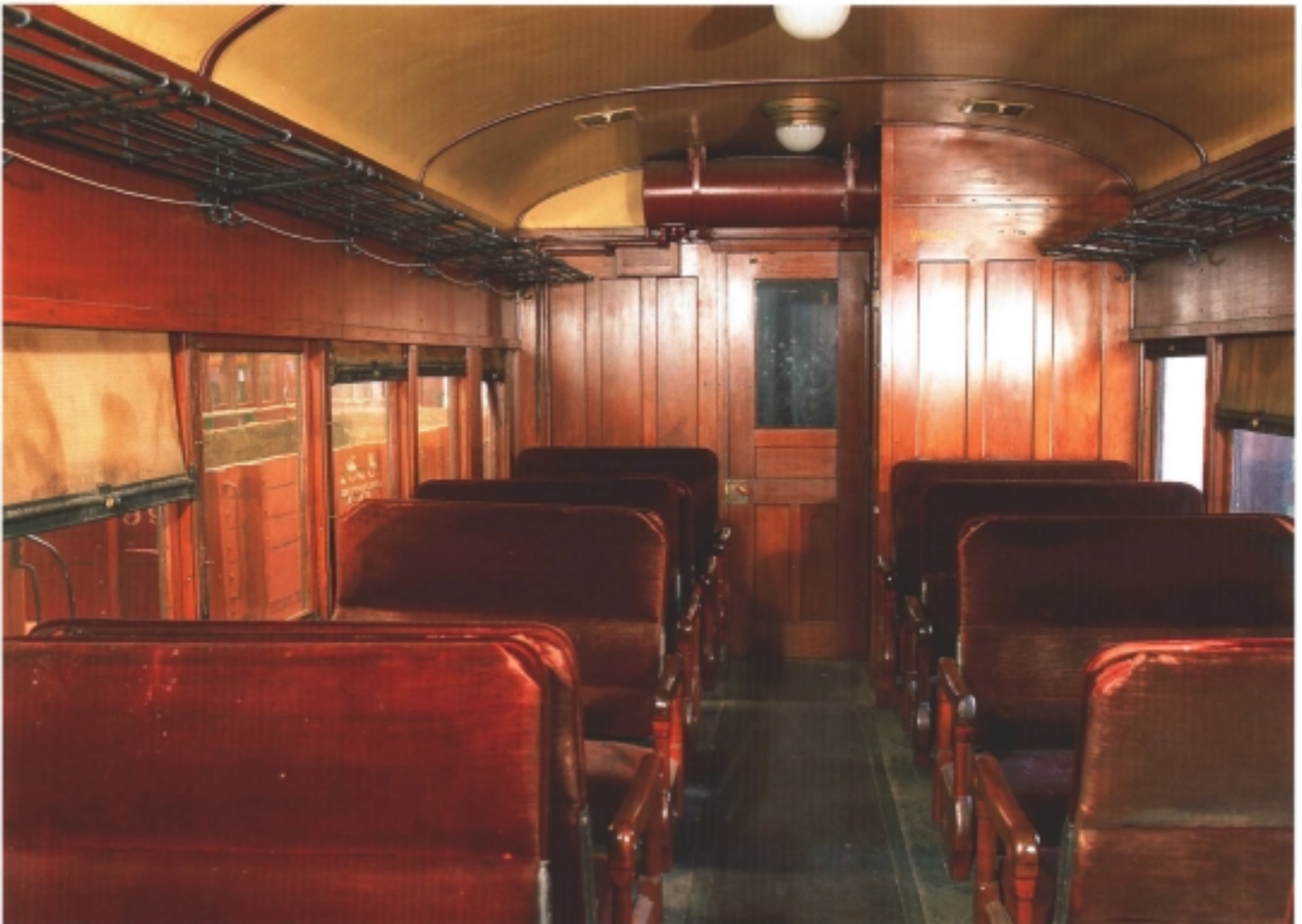
MW 31's main passenger compartment presently seats 26, but the original floor plan shown earlier indicated an off-center aisle, thereby accommodating 32. The seats apparently changed after 1931; they now are the same width on both sides of the aisle. Air vents in the ceiling were connected to ten "Garland" ventilators mounted on the roof to promote fresh air ventilation. Paul Swanson photo, August 26, 2002.
