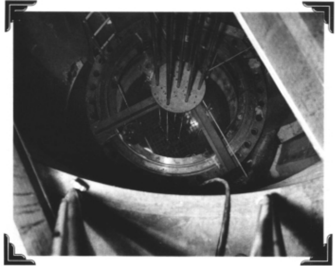
The pressure vessel from above, showing reactor control rods being inserted.
